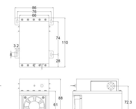
Outline wit heatsink and Fan in default Customer can remove the heatsink and Fan if using their own heatsink system.
